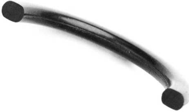
Fig. 10.8 Damage pattern caused by high compression set
