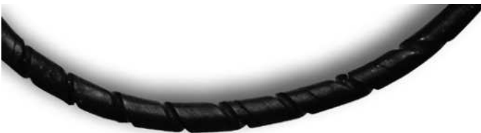
Fig. 10.9 Twisted O-ring with spiral markings
