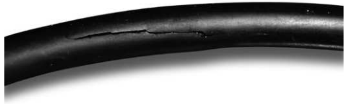
Fig. 10.11 O-ring damaged by explosive decompression
