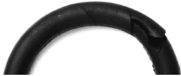
Fig. 10.10 Twisted O-ring with cuts in surface
